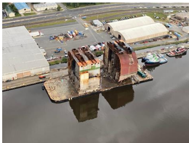
Loaded with Sections Three and Six of the Golden Ray wreck, the Barge Julie B continues sea fastening on Friday, Oct. 8, 2021, at Mayor's Point Terminal in preparation to transit the sections to Louisiana. St. Simons Sound local response facility for partial dismantling.
