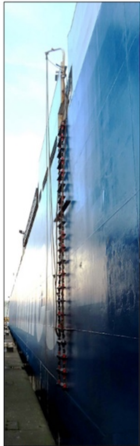
Figure 3: Finnhawk 's pilot ladder
