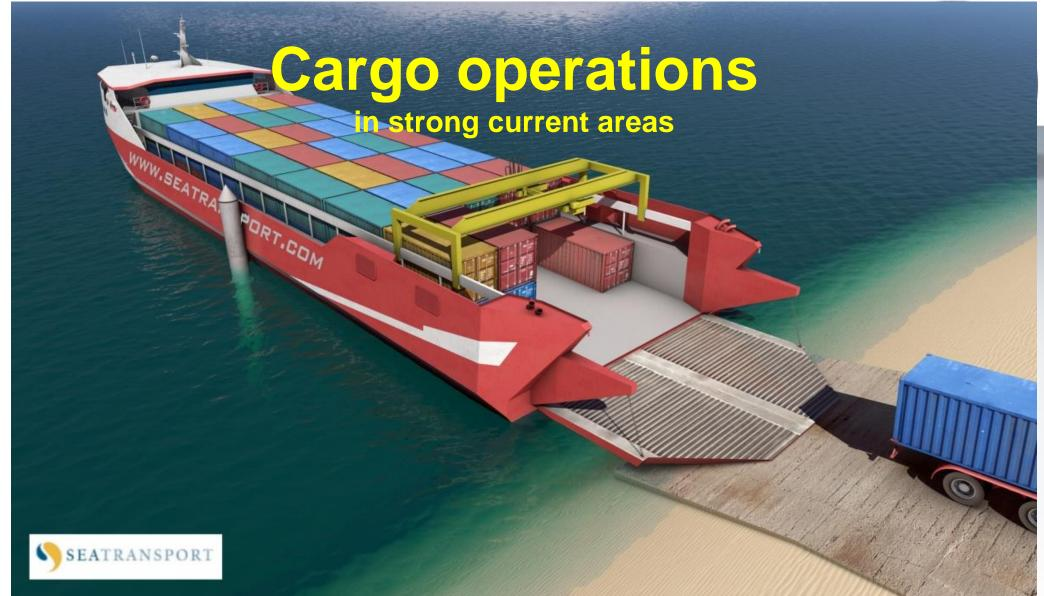
The container, roro or bulk cargo can be handled easily in this mooring arrangement during normal tidal flows
