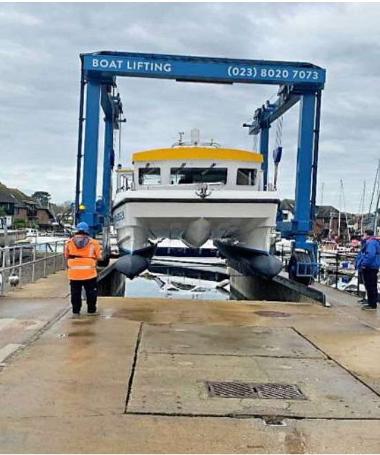
Relaunch on March 31st Whilst still in the slings, Marlin Marine had the honour of starting their new engines for the first time since installation. We headed out into perfect conditions in Southampton Water and under the watchful eyes of Marlin's engineers, she was put through her paces, ultimately winding up to full speed. With no water or exhaust leaks and running sweetly throughout, sea trials were declared a success.
