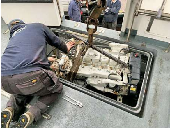
Port engine being removed
