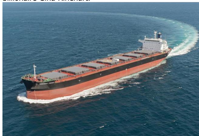
**The recently delivered bulk carrier, *MV Harvest Frost*, is the first vessel of its size to use MHI's proprietary Mitsubishi Air Lubrication System (MALS), which reduces the drag between the vessel hull and seawater by blowing air bubbles produced at the vessel bottom. Photo credit: MHI**
