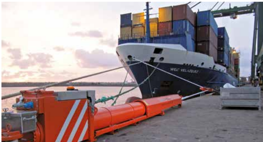
A Shoretension mooring unit by Dutch company KRVE and in growing use in Australia.
